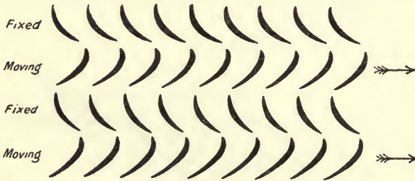
FIG. 99.—Arrangement of blading for Parsons turbine.
